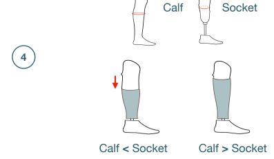
If the circumference of the prosthetic socket at its widest point is similar to the calf circumference (or greater), the Cover height should be as low as possible. It is important to remember that placing the Cover on the socket increases its circumference and may not look good together with the healthy leg.
